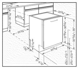
Machine heights of 35" - 37" (889-940 mm) cannot be obtained using the supplied legs.
